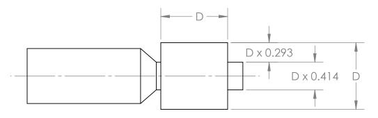
Turn a cylinder with its length the same as its diameter. The tenon diameters should be the large diameter times 0.414.
