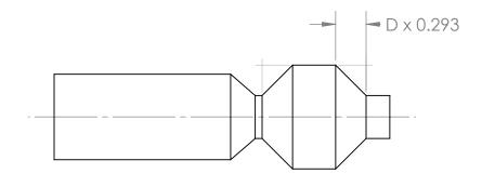
Make a mark 0.293 times the large diameter from each end and turn a straight line connecting it with the edge of the tenon (both ends).
