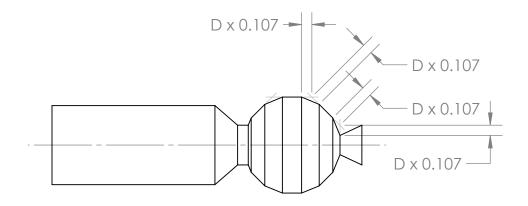
From each of the new edges, mark a line 0.107 times the large diameter on each side. Connect those two marks with a straight line.
